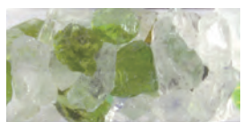
Grade 3 equivalent to 6mm gravel
